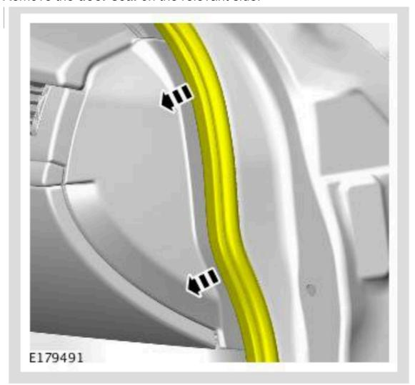
Position the door seal to one side.
